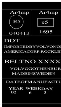
*Label on seatbelts with seatbelt tensioner*
